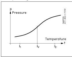
In this case the charge consists partly of a superheated gas and partly of a solid having a large adsorption surface.
