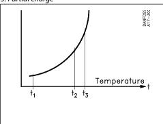
Partial charge is used in RT units having a range lying higher than ambient temperature.
