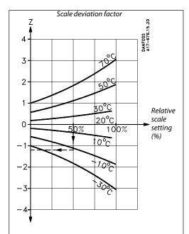
Curves for different ambient temperatures. 0% ~ lowest scale setting temperature, 100% ~ highest scale setting temperature.
