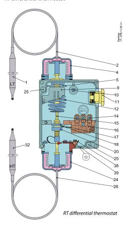
An RT differential temperature control contains a single-pole changeover switch that makes or breaks depending on the temperature difference between the two sensors of the unit.
