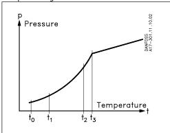
Here the interdependence between the pressure and temperature of saturated vapour is utilized, i.e. the element is charged with saturated vapour plus a small amount of liquid.
