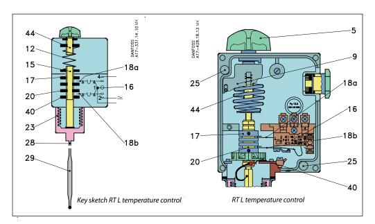
RTL temperature controls are fitted with a switch (17-4032) with an adjustable neutral zone. This enables the units to be used for floating control. The neutral zone switch contact arms (18a) and (18b) are operated by the spindle guide bushes (17) and (20). The upper guide bush (17) is fixed
